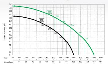
Blizzard has been tested to perform under long ducting, and the resulting chart shows that the airflow (with 10m ducting) still remain reasonably well at around 50% of peak extraction. \*Testing is done based on 150mm duct diameter.
